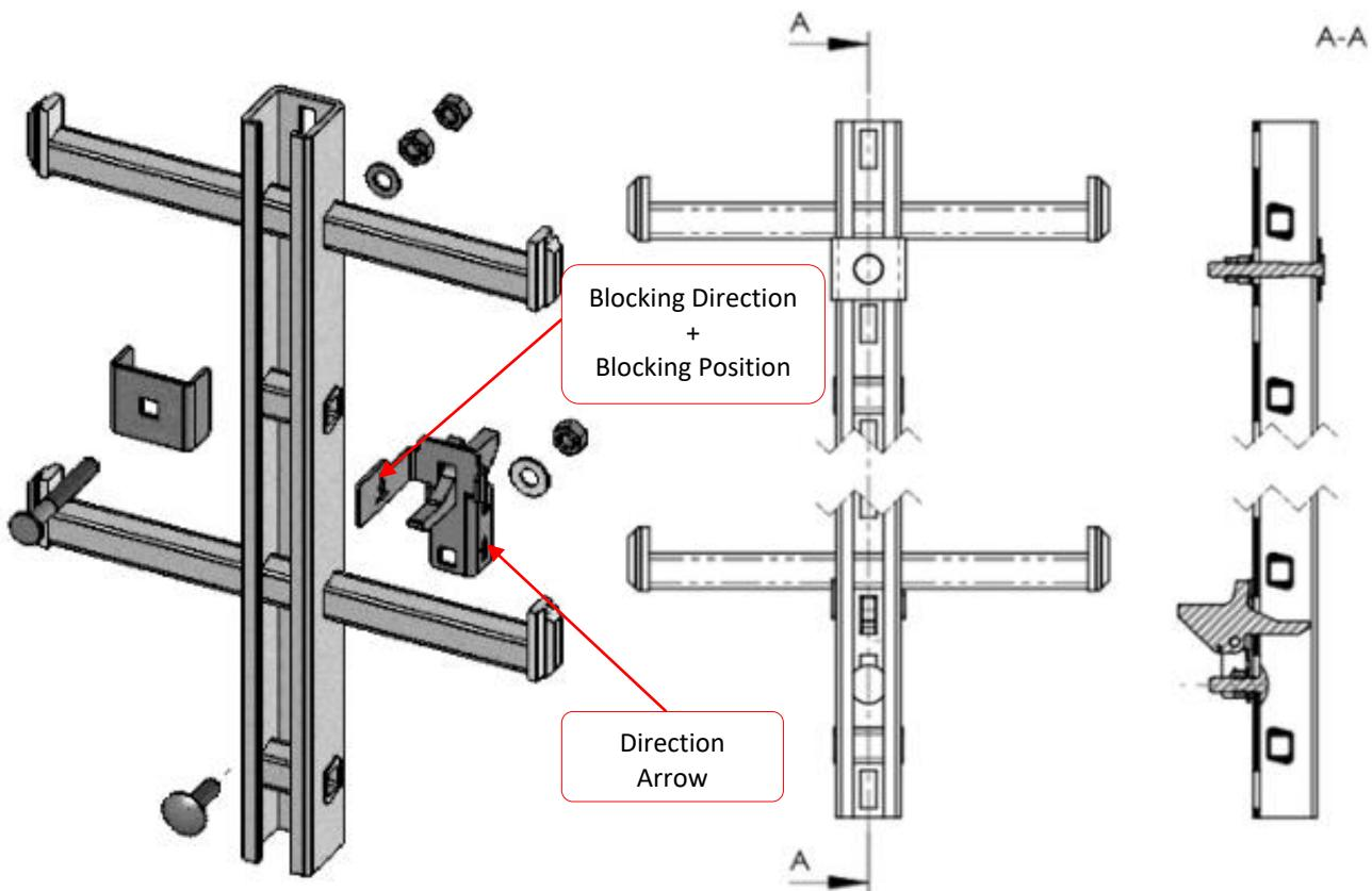
Picture shows climb way with openable bottom end stop and rigid top end stop
