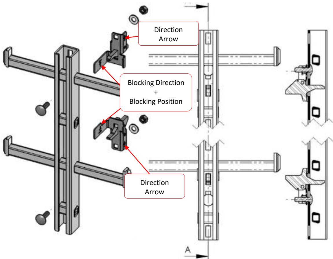
Picture shows climb way with openable bottom end stop and openable top end stop
