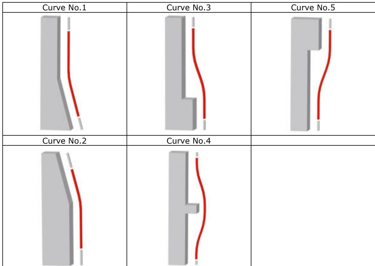
**ATTENTION !** The Twinstop® fall arrester can be used in rails at inclination + 20° or -20° reclined, as well as a sidewise inclination (left and right) of 15°.
