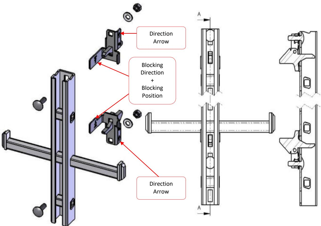
Picture shows climb way with openable bottom end stop and openable top end stop
