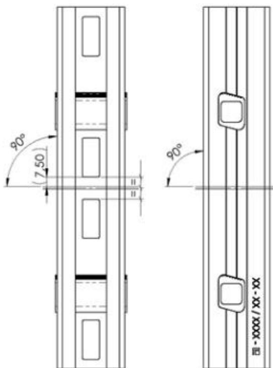
The cut has to be rectangular to the rail. If a segment in the between of a system installation, has to be shortened it has to be always in 140 mm steps and centric between the two slots which are near to each other.
